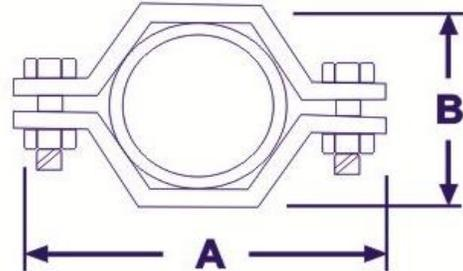
**HIGH TEMPERATURE HANGERS MADE FROM AISI-304 STAINLESS STEEL COLLARS/SLEEVES CAN WITH STAND TEMPERATURES OF 325 DEGREE F**
